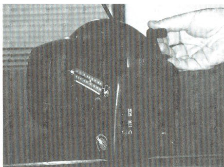
BayGen's "Freeplay" wind-up radio receives AM and FM. Another BayGen model also receives shortwave broadcast signals.
