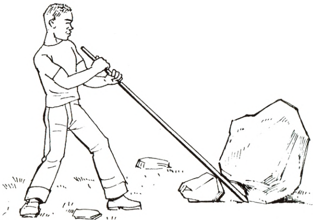
Example of a simple lever being used-man raising rock with a long stick and a small stone.
